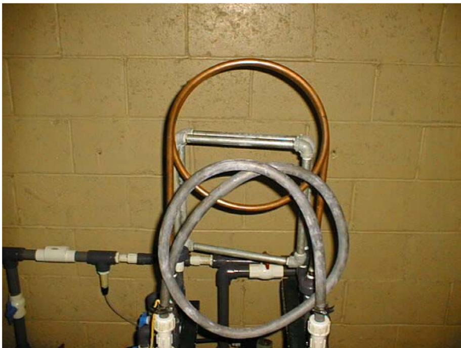
*A close-up picture of the lead, copper, and galvanized iron pipe loops.*
