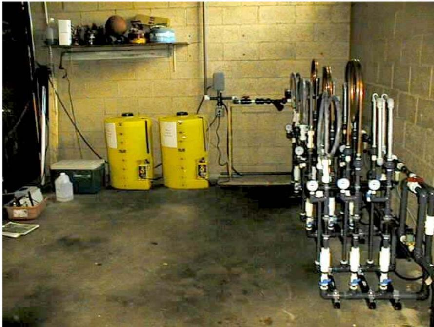
*Side view of the pipe loop apparatus at the Village of Dane. Along the back wall are chemical tanks and pumps for sodium hypochlorite and potassium orthophosphate. The timer which controls the drain line solenoid valve and the chemical pump electrical outlet is the rectangle on the back wall.*
