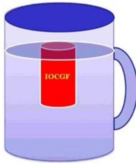
Figure 10. Schematic design for IOCGF pitchers used in field tests
